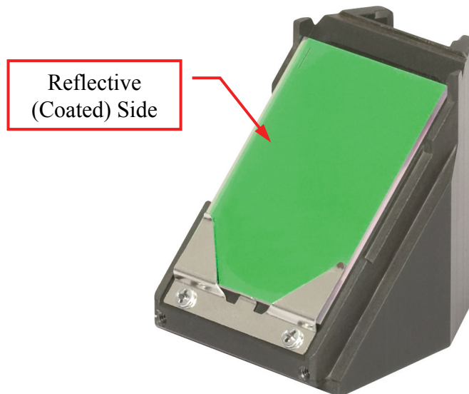
Figure 6. The dichroic mirror mounted in the emitter half cube
