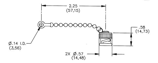
MATERIALS: Body – Nickel Plated Brass Gasket – Silicone Rubber
