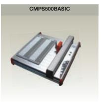
The CMPS500BASIC unit is an A4 size auxiliary plotter and has to be connected to a computer via a USB connection. It is a high speed plotting device and enables plotting of different markers in one setting. The marker fixture and the plotter pen have to be inserted before commencing the plotting operation. The base unit is primarily controlled through a computer with the help of CMPS software.
