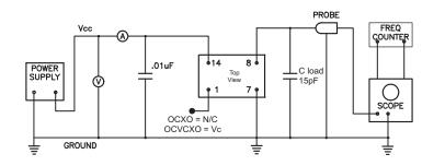
**BOC1 Series Test Circuit**
