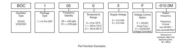
BOC10503F-010.0M = 14 Pin DIP package, ±50 ppb, 0 to 70°C, 3.3 Vdc, LVCMOS Output, OCXO, Output Frequency 10.0 MHz
