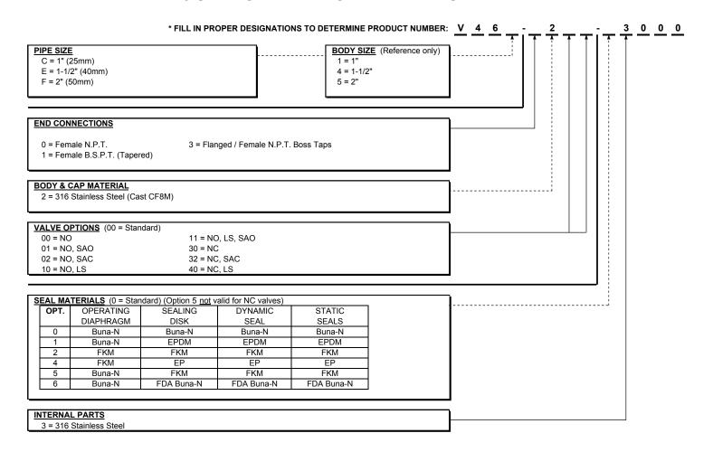
\* To create a valve number replace each "\_" with the proper number or letter for the feature you desire. For example, a 1" NPT Stainless Steel Valve Model V461 with Normally Closed and Spring Assist Closed Options is designated as a V46C-0232-03000.
