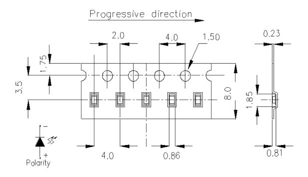
**Note:** The tolerances unless mentioned are  $\pm 0.1$ mm, unit = mm
