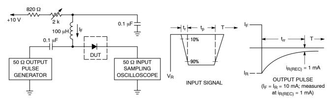
Notes: 1. A 2.0 k $\Omega$  variable resistor adjusted for a Forward Current (I<sub>F</sub>) of 10 mA. 2. Input pulse is adjusted so I<sub>R(peak)</sub> is equal to 10 mA.
