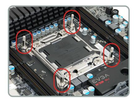
After these posts have been installed, mount the EVGA Superclock Cooler as instructed in Intel® mounting guide.
