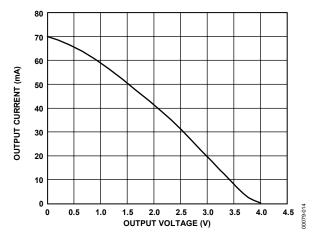
Figure 19. Output Current vs. Driver Differential Output Voltage
