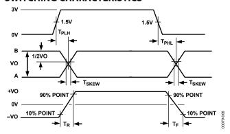
Figure 11. Driver Propagation Delay, Rise/Fall Timing
