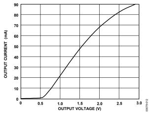
Figure 17. Output Current vs. Driver Output Low Voltage
