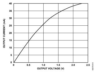
Figure 15. Output Current vs. Receiver Output Low Voltage
