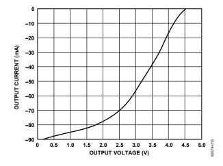
Figure 18. Output Current vs. Driver Output High Voltage
