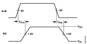
Figure 12. Receiver Propagation Delay
