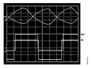
Figure 20. Driving 4000 Ft. of Cable
