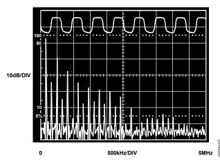
Figure 27. Driver Output Waveform and FFT Plot Transmitting at 150 kHz
