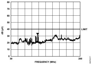
Figure 22. Radiated Emissions
