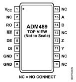
Figure 5. ADM489 16-Lead TSSOP Pin Configuration
