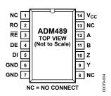
Figure 4. ADM489 14-Lead PDIP/SOIC Pin Configuration
