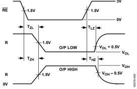
Figure 14. Receiver Enable/Disable Timing
