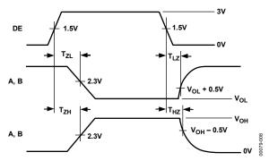
Figure 13. Driver Enable/Disable Timing
