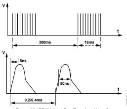
Figure 25. IEC1000-4-4 Fast Transient Waveform
