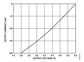
Figure 16. Output Current vs. Receiver Output High Voltage
