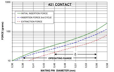
The insertion/extraction/normal force characteristics above were derived using 0,76 micrometers gold plated contact and polished steel gauge pins having a bullet-shaped tip.
